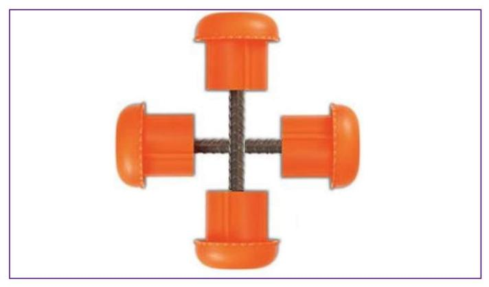
Our Rebar Safety Caps can be used to protect construction workers from the danger of being pierced by protruding rebar. Rebar sticking out from pillars or columns on a slab present the real danger of piercing workers who may trip and fall on site. Rebar sticking out from the sides of slabs could cause workers to loose an eye.
