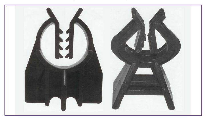
Plastic Rebar Spacers with Rebar clip are similar to rebar chair spacers and are used to support rebar or mesh on a deck. The wide base of these rebar clips prevent the clips from tipping over. The design ensures freeflow of concrete and minimal contact with the concrete formwork.
