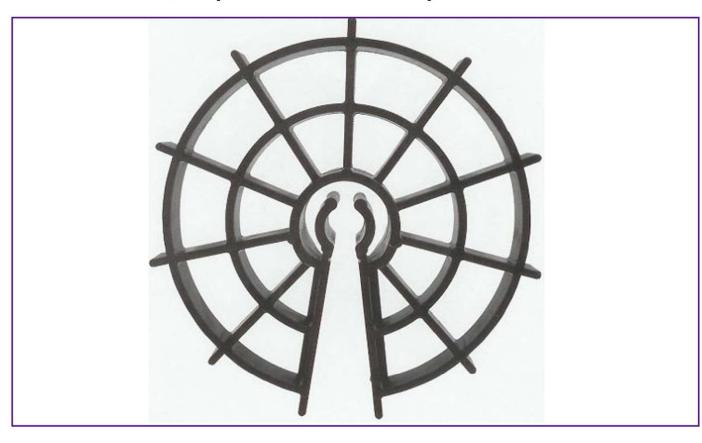
Plastic Wheel spacers (Circular spacers) are used to ensure consistent concrete cover for columns, cages and walls inside the concrete shutter or precast formwork. Plastic Wheel spacers help to ensure the centralisation of rebar inside the shutter or precast formwork. The notched outer rim of the plastic wheel spacers ensure minimum contact with the shutter or precast formwork.
