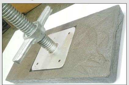
Our Base Jack Sole Boards (Also called Toe Board) are used to support the base jack. It stops the base plate from slipping on the surface bed and also stops it from, sinking into the surface bed. The Base Jack plate fits into a specially crafted square inset, to ensure that the Base Jack Plate fits properly into the Base Jack Sole Board / Toe Board.
