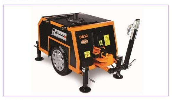
This Lombardini Diesel Engine driven mobile rebar cutter and bender, with an electric starter, will cut and bend rebar up to a diameter of 32mm. Cutting and bending is achieved through a hydraulic system. It requires minimum maintenance. It is easy to use and comes with tooling to do stirrup bending as well as other standard bending operations. This compact self sustained mobile rebar cutter and bender allows for movement over vast distances and into remote areas.
