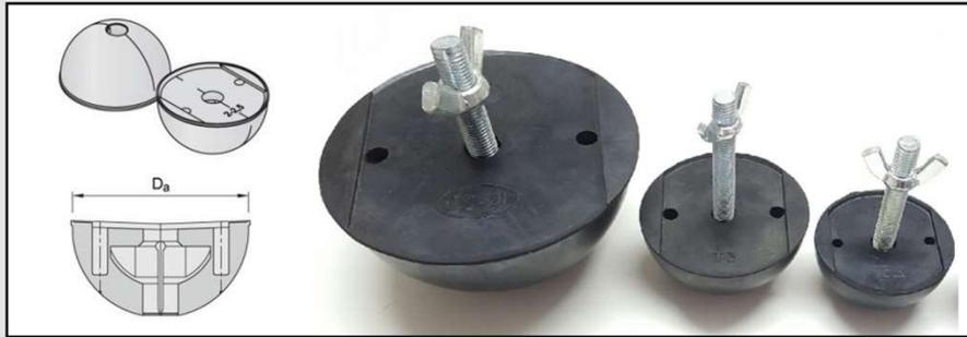
The Rubber Recess Formers must be used to fix the Spherical Head Anchors (T Anchors) to the formwork. This ensures simple and secure locating of the anchor in the concrete element and leaves the anchor ready for the correct universal head lifting clutch.
