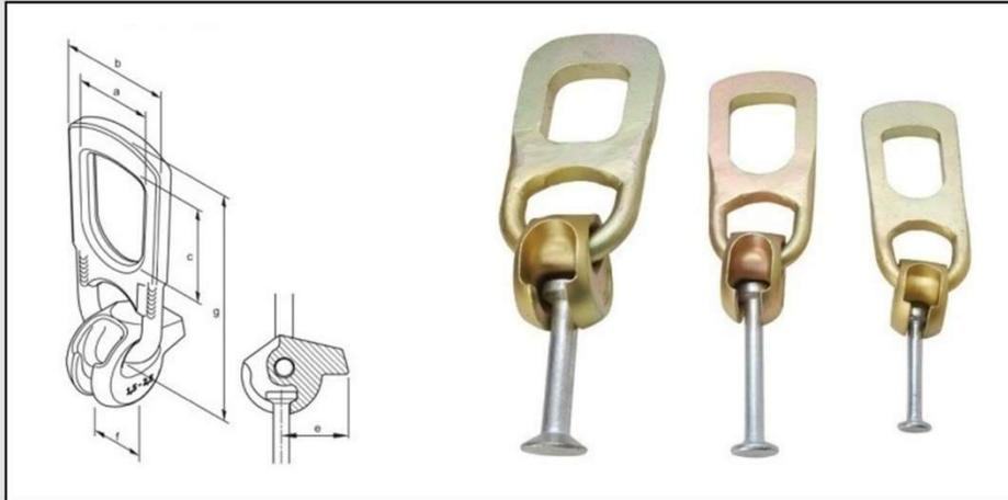
The capacity loads are axial with breakage safety factor equal to 5 for all types of lifting clutches (1,3 ton up to 32 ton). The Spherical Head Lifting Clutch comes in 6 different load groups. 1,3 to 32 ton, to suit the load carrying range of ALL TYPES OF LIFTING ANCHORS with spherical-heads.
