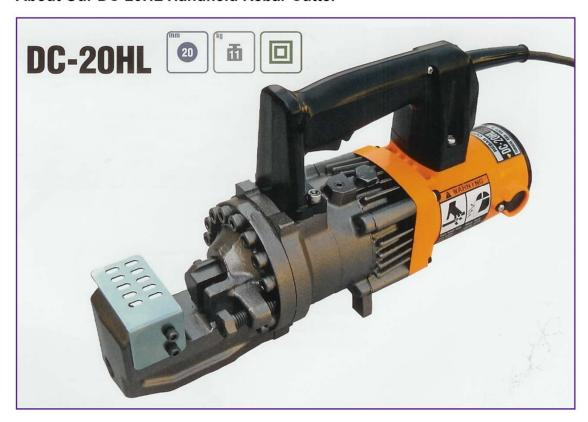
Our DC-20HL handheld rebar cutter is a popular heavy-duty tool for general use. The DC-20HL helps save valuable manhours by cutting from 4mm up to 20mm rebar within 4 seconds at the job site or in your shop. The DC-20HL has a newly developed balanced armatures and hardened piston for long life. Relatively light weight at 11.5 kilograms.
