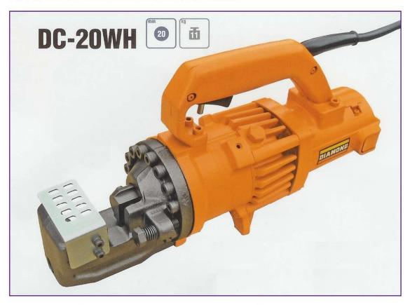
Our DC-20WH handheld rebar cutter is a popular heavy-duty tool for general use. The DC-20WH saves valuable manhours by cutting from 4mm up to 20mm rebar within 3 seconds at the job site or in your shop. The DC-20WH has a newly developed balanced armatures and a hardened piston for long life. Relatively light weight at 11.5 kilograms.
