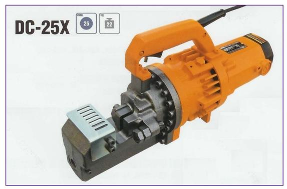
Our DC-25X handheld rebar cutter is a popular heavy-duty tool suited to larger construction jobs or rebar fabrication shops. The DC-25X helps save valuable man-hours by cutting from 4mm up to 25mm rebar within 5 seconds at the job site or in your shop. Weighs 22.5 Kilograms.
