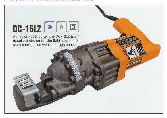
Our DC-16LZ handheld rebar cutter is a compact, medium-duty rebar cutter. The small head of the DC-16LZ will fit into tight spots. The DC-16LZ handheld rebar cutter helps save valuable man-hours by cutting from 4mm up to 16mm rebar at the job site or in your shop. It takes the DC-16LZ 2 seconds to cut 16mm rebar. Light weight at 6 kilograms.
