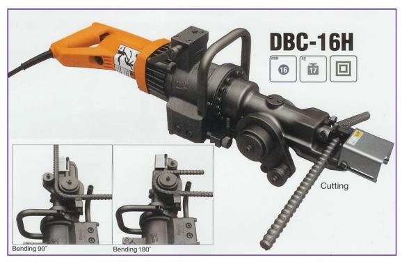
Our heavy duty, convenient DBC-16H handheld combination rebar cutter and bender can cut and bend rebar up to 16mm. The DBC-16H enables you to cut 16mm rebar within 2.5 seconds and then bend it up to 180 degrees within 5.5 seconds whenever and wherever the need arises. The rebar cutting or bending option is selected by simply turning a lever. Weighs 17 kilograms.
