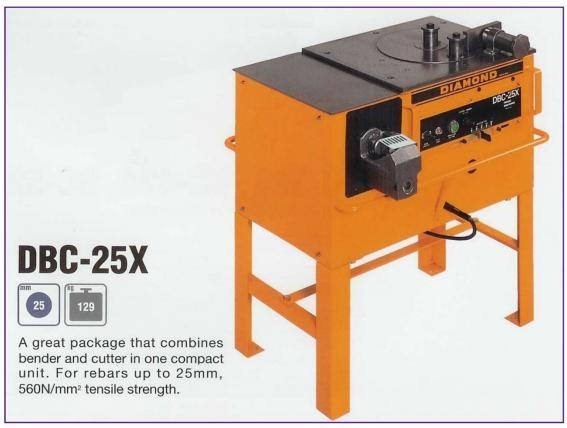
Our compact DBC-25X portable rebar cutter and bender combines rebar cutting and bending in one unit. The DBC-25X enables you to cut up to 25mm rebar within 5 seconds and then bend it up to 180 degrees within 6 seconds whenever and wherever the need arises. This single phase unit can run off a generator for deployment at remote sites. Weighs 129 kilograms.
