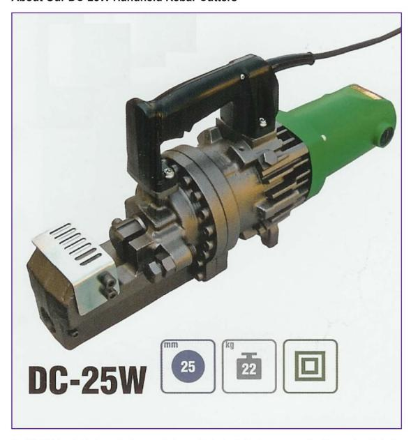
Our DC-25W handheld rebar cutter is a popular heavy-duty tool suited to larger construction jobs or rebar fabrication shops. The DC-25W helps save valuable man-hours by cutting from 4mm up to 25mm rebar within 4 seconds at the job site or in your shop. Weighs 22.0 kilograms.
