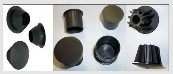
Rebar, Mesh and Construction Supplies (Pty) Ltd supplies a wide range of Formwork accessories such as Shutter buttons, shutter plugs, Vario button to the construction and related industries. Our shutter buttons and plugs are used to plug redundant or unused holes Formwork panels. Shutter buttons or plus are put into the holes by simply tapping them in with a hammer or pushing them in by hand.
